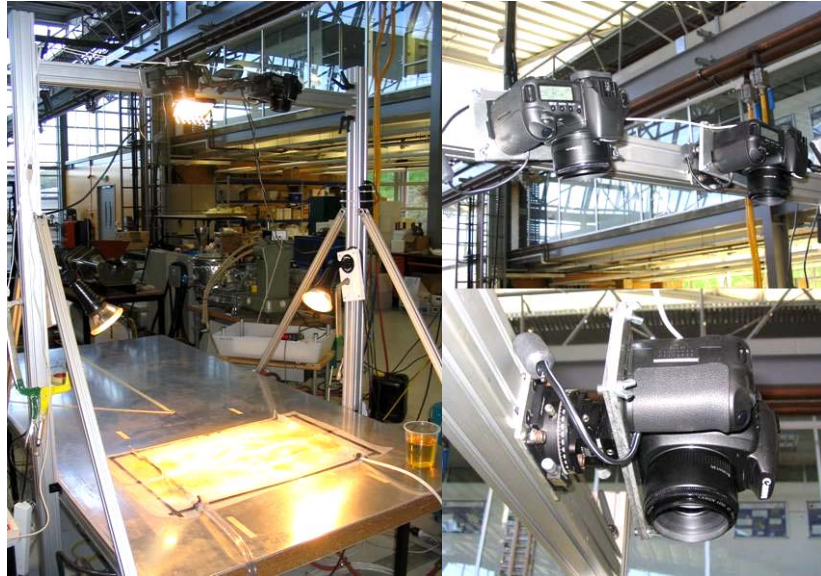
Figure 5: Details of the stereophotography rig.
