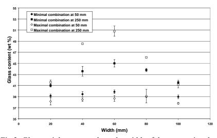
Fig.3: Glass weight content along the width of the composite plates.
