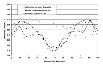
Fig.5: Fibre orientation profiles through-the-thickness of the injection moulded part
