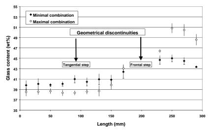
Fig.2: Glass weight content along the mid-axis of the composite plates
