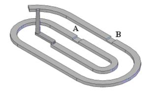
Fig. 2. Cut-sections parallel to the plane of flow at locations A & B for analyzing the state of fiber orientation in the mid-plane (Core layer)
