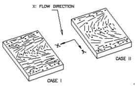
a. Schematic pattern of fiber orientation at location A (Cases I & II)
