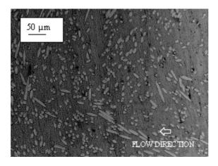
c. Higher degree of out of plane orientation of fibers at location A<sub>ii</sub> (Case III)
