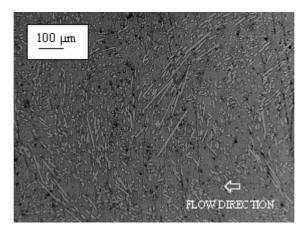
c. Higher degree of transverse orientation of fibers at the centerline (Case II)
