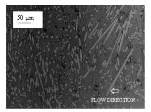
b. Higher degree of in-plane transverse orientation of fibers at location A<sub>i</sub> (Case II)
