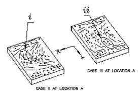
a. Schematic pattern of fiber orientation at location A (Cases II & III)
