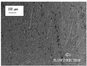
c. Higher degree of transverse orientation of fibers at location B (Case III)
