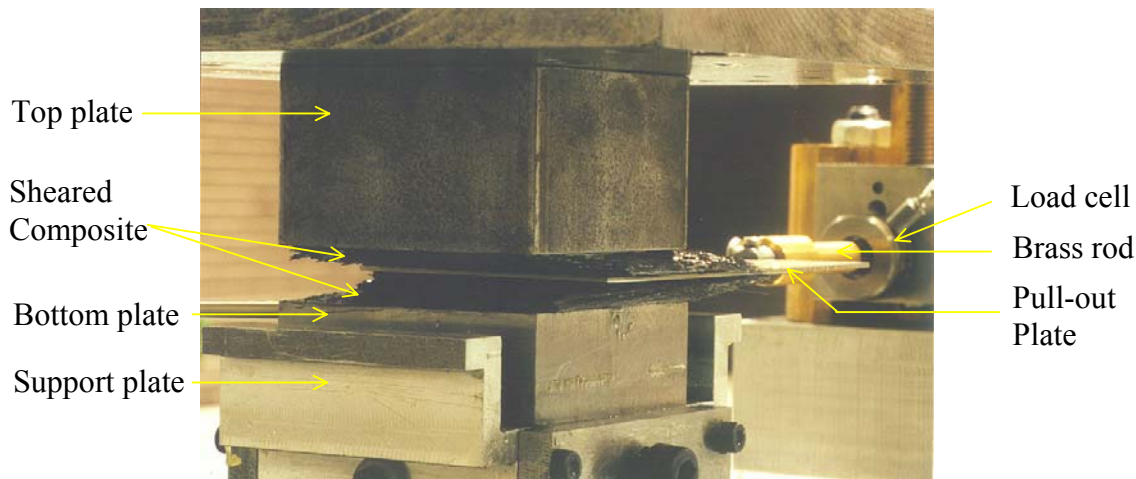
Figure 2: Photograph taken of a typical test in progress.
