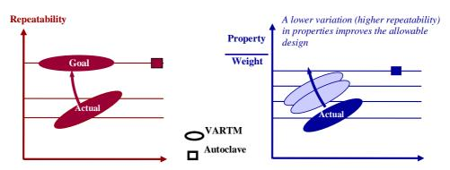
Figure 1: VARTM has the potential to reduce cost with equivalent repeatability compared to autoclave processing
