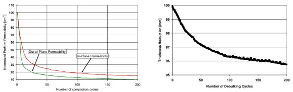
Figure 2: Debulking alters the thickness and permeability of the incoming reinforcement
