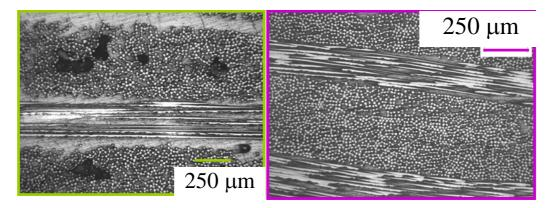
Figure 4: Vinyl ester part on the left shows high void content versus below 1% for the epoxy part
