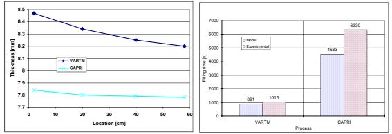
Figure 3: The CAPRI process improves fiber volume fraction and dimensional tolerances while increasing processing time
