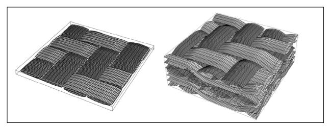
Figure 2 FE mesh for surfaces of yarns of one layer of woven fabric and a laminate
