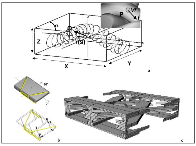
Figure 1 (a) Set of cross-sections defining a yarn in a unit cell, properties of fibres near point P; (b) Quadriaxial NCF, orientation of the fibres in the plies 0°/-45°/90°/45°:) Full geometrical model with stitching. Note a "channel" in the first 0° ply and slab representation of a ply with -45° "cracks". ABCDEF – vertices of the upper polygon of one of the slabs; (c) Example of the pore structure of biaxial NCF
