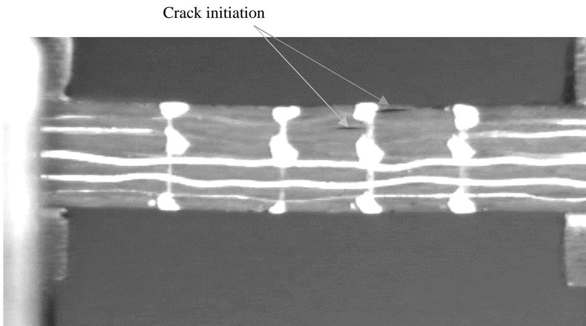
Figure 4. Picture showing the initiation of delamination at the interface of the wrinkled and angle plies in the specimen. (Note the white dots are marked on the specimen edge to monitor strains during the test)
