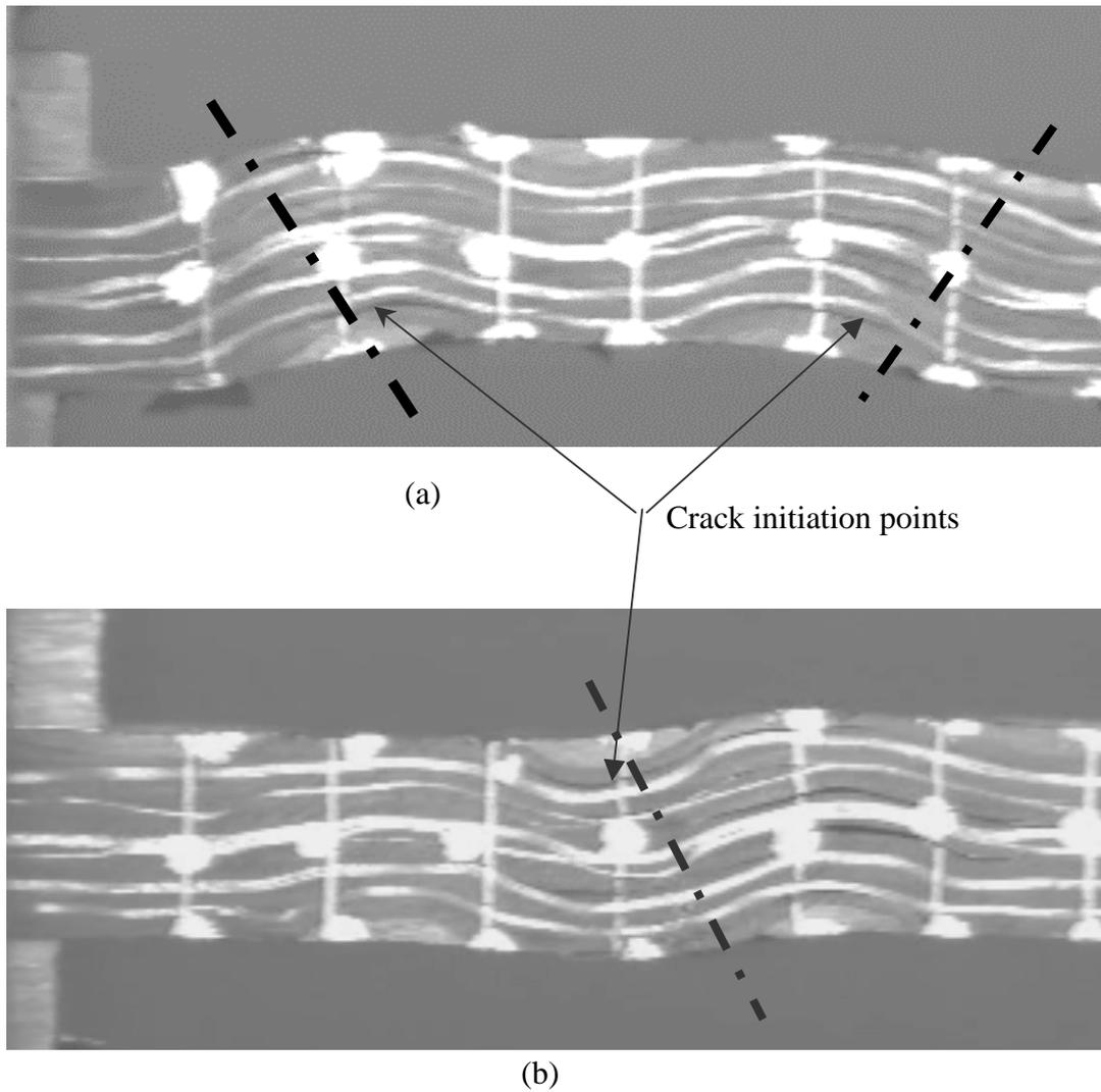
Figure 5. Different types of failure pattern observed in the samples (a) with delamination initiation at two locations and (b) with one initiation location. The dashed line denotes the general plane of failure corresponding to maximum fibre misalignment.
