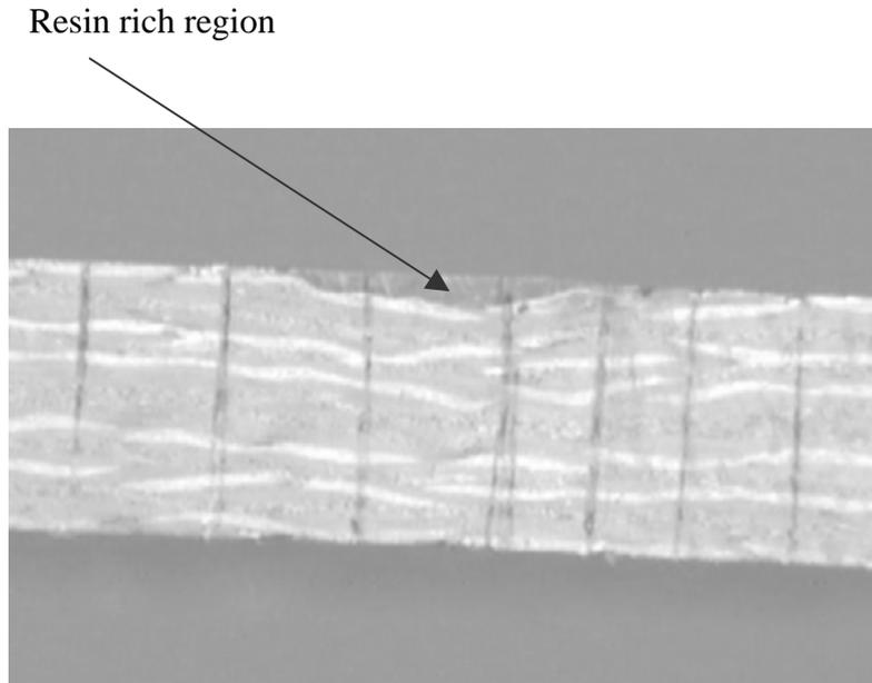
Figure 3. Resin richness simulated on the top surface of the specimen
