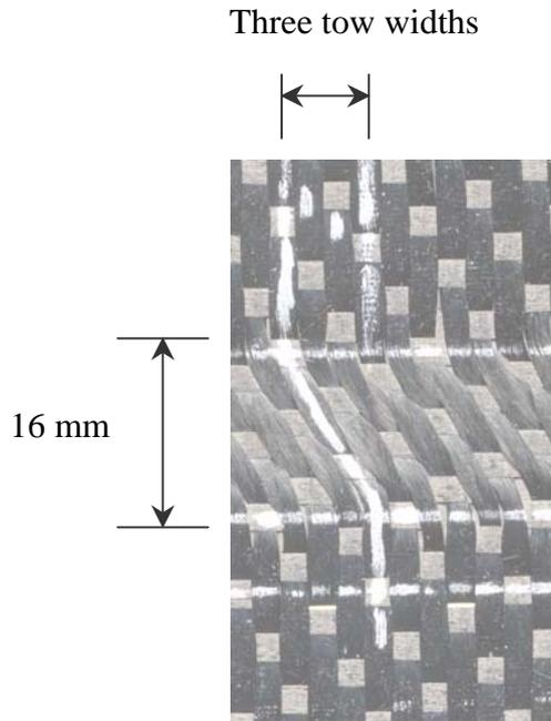
Figure 1. Picture showing in-plane fibre tow distortion in simulating wrinkling of fabric.
