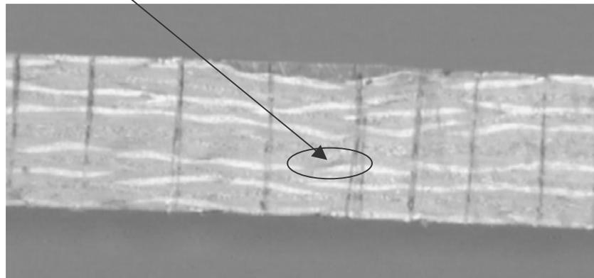
Figure 6. Schematic diagram (a) with picture showing initiation of delamination in (b) at the interface between the straight and deformed layers and subsequent propagation
