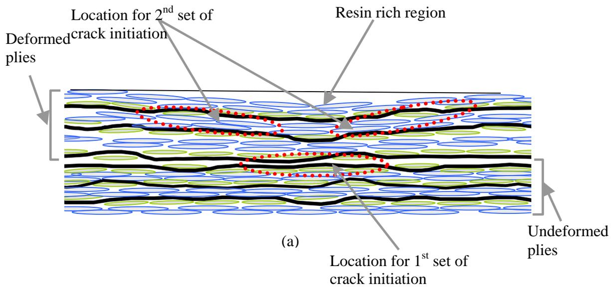
Initiation of 1<sup>st</sup> set of cracks at the interface between the deformed and undeformed layers
