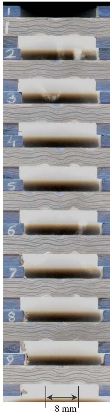
Figure 2. Out of plane fibre distortion simulating fabric folding .
