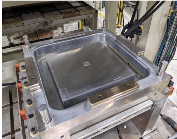
NRC flat plate tool 350x350 mm
