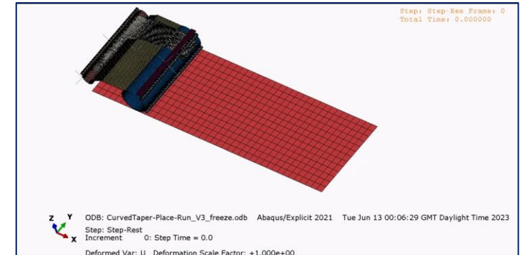
Placing curve tapered ply (3 x 1.2 m)
