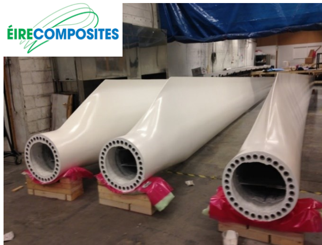
13.0m wind turbine blades manufactured by ÉireComposites (Ireland)
