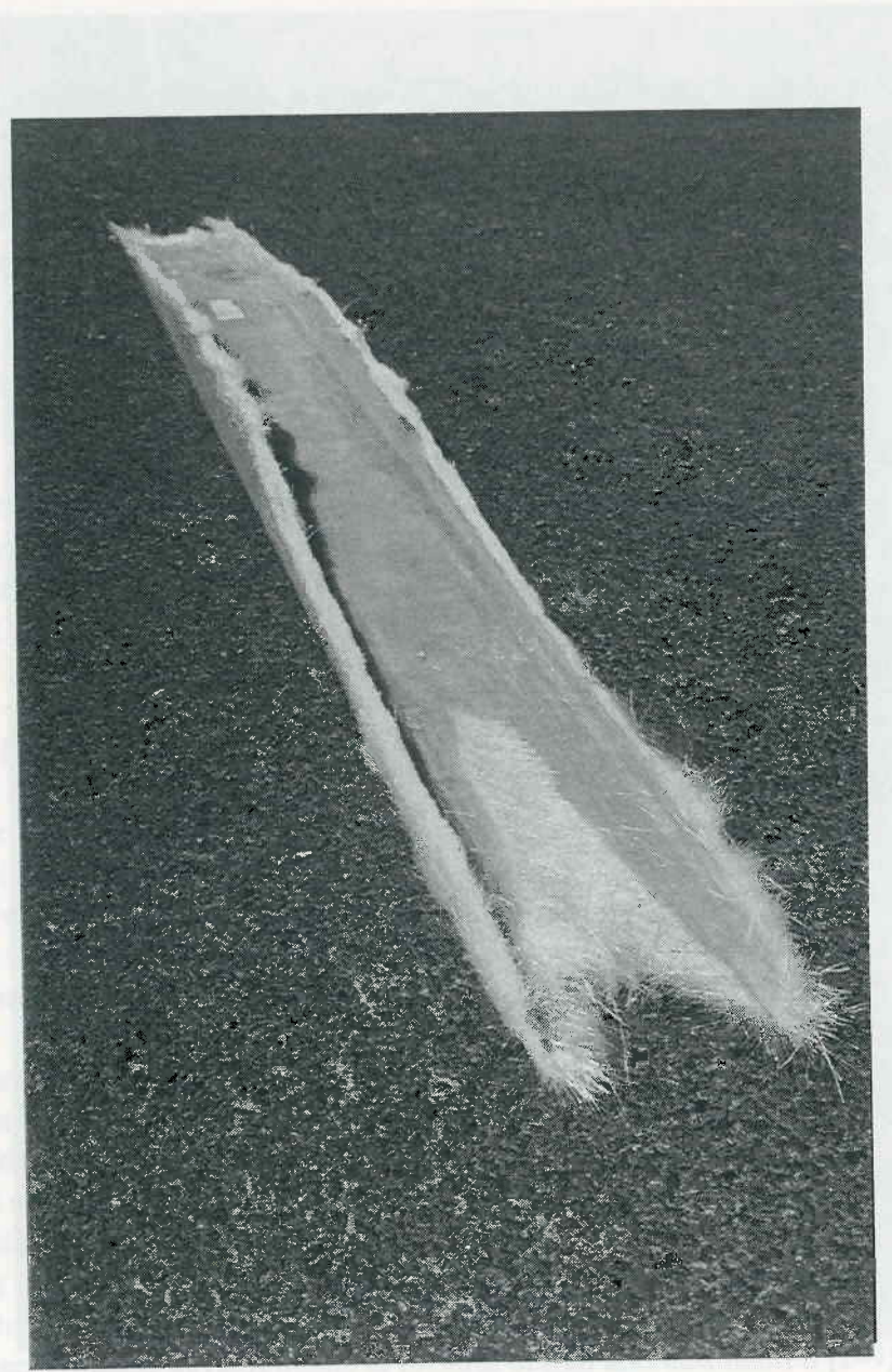
Partially Filled beam where the flow front may be seen
