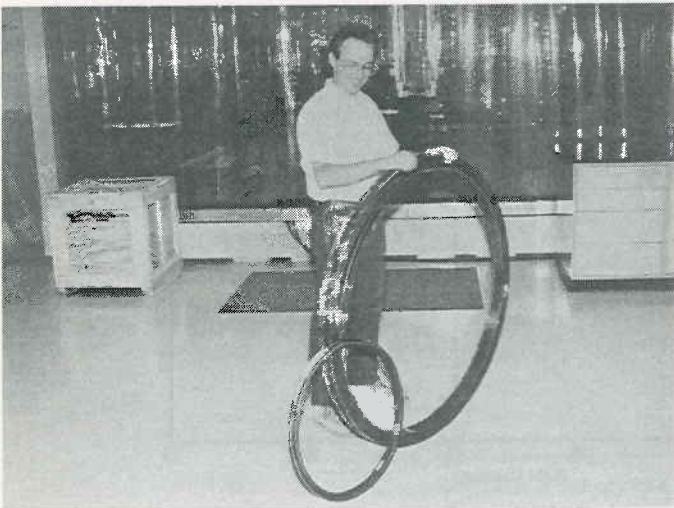
Figure 11 - Stamped, Co-Consolidated, 1,22m Dia. and 61 cm Dia. AS4/APC-2 Stiffeners
