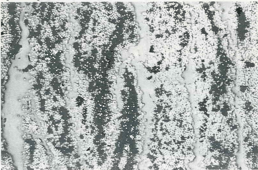
Fig. 12: Laminate without preheating. The micrograph shows the different winding layers and voids and thus a poor consolidation of the laminate.
