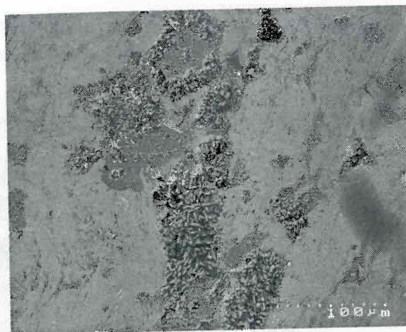
Figure 4 SEM back scattered image of the cross section of AMC sample made by consolidating the powder mixture of Al alloy powder and \text{Al}_2\text{O}_3 powder.
