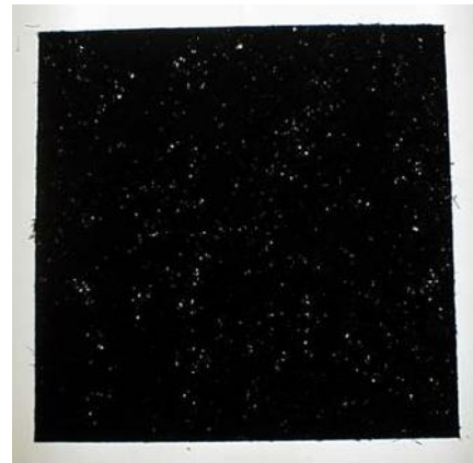
Fig. 2: Carbon Roving A @ 1000 g/m 2
