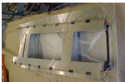
Figure 7: Mold with preforms (left) and mold sealed with preshaped bags and closing plate (right)
