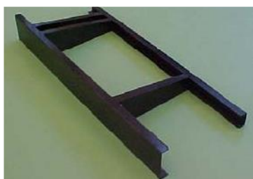
Figure 8: The integrated rib-spar structure (left), a skin (middle) and a leading edge rib (right)
