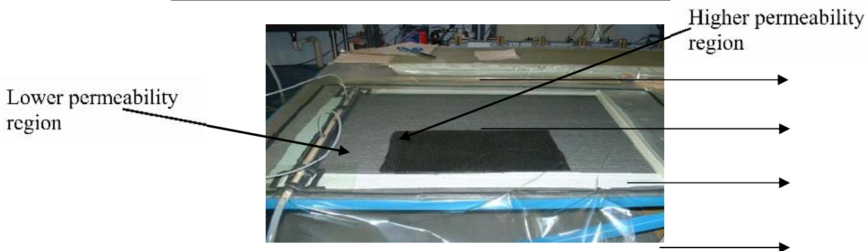
Figure 3: Preform pattern and modified set up using segmented injection line
