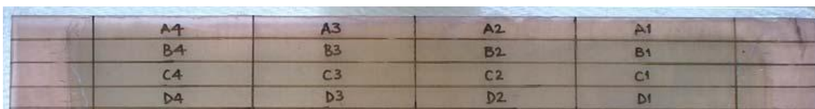
Figure 5. Specimen to be cut from a composite part along the upper edge.
