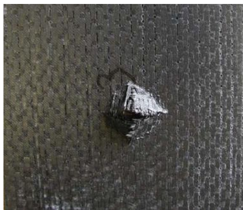
Figure 5 Tensile face of typical impacted sample.
