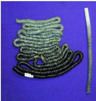
Figure 3. Graded polymer composites manufactured using the TSE process
