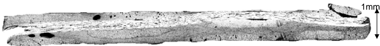
Figure 1 CF/APLC12 plate cross section (before heating/stamping): porosity =3.5%
