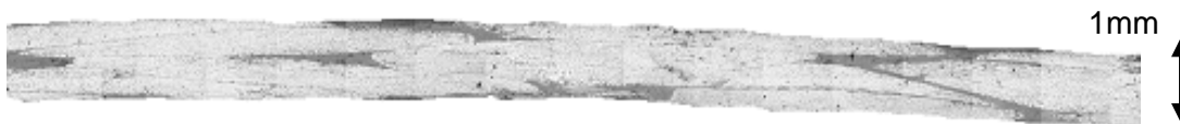
Figure 4 CF/APLC12 stamped sheet cross-section (preheat temperature = 200°C, stamping rate = 166mm/s, 2% activator level) void content = 3.1 %
