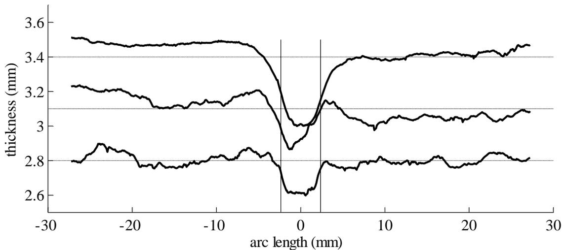
Fig. 7 Influence of injected quantity upon the final thickness profile.
