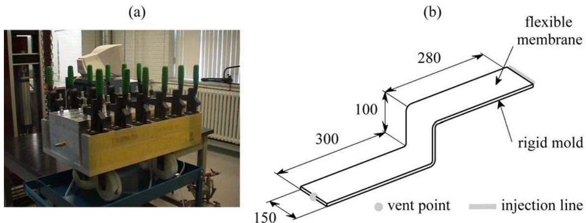
Fig. 2 Implementation of the flexible injection process for curved part manufacturing: (a) experimental mold and (b) geometry of the part (dimensions in mm).
