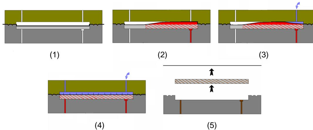
Fig. 1 Main steps of the flexible injection process.
