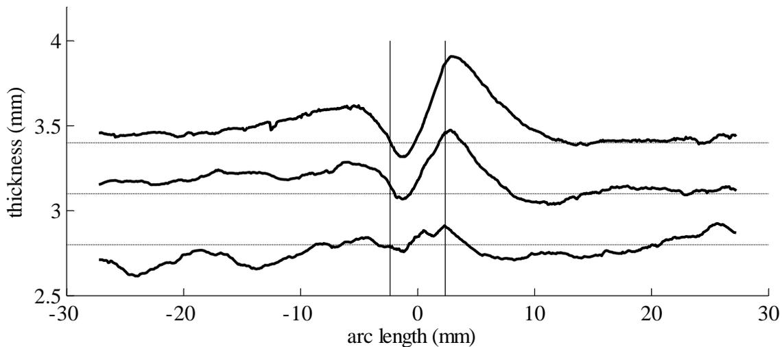
Fig. 9 Thickness profiles illustrating the displacement of the resin-rich zone.
