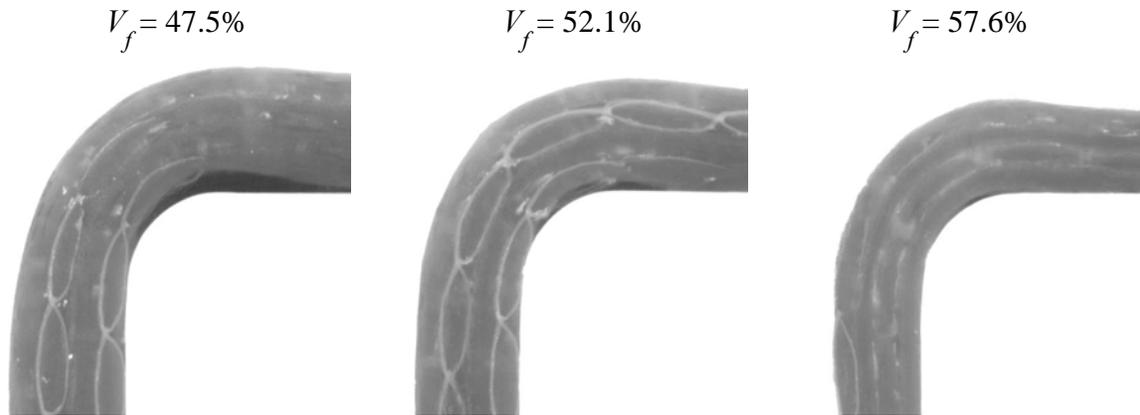
Fig. 8 Resin-rich zone creation induced by poor preform dimensioning.
