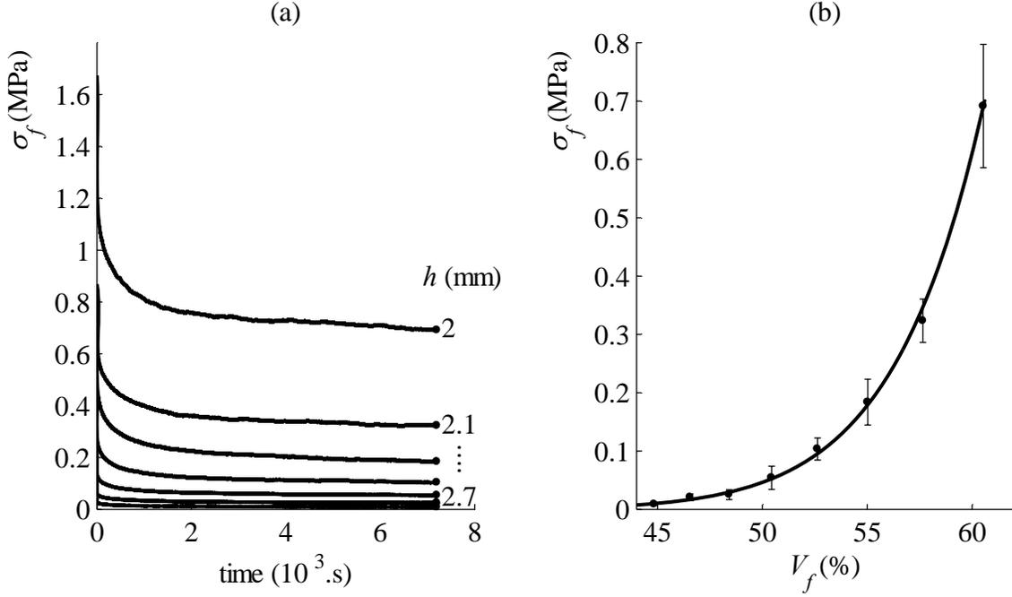
Fig. 5 Characterization of the fiber preform: (a) relaxation curves and (b) compaction law.
