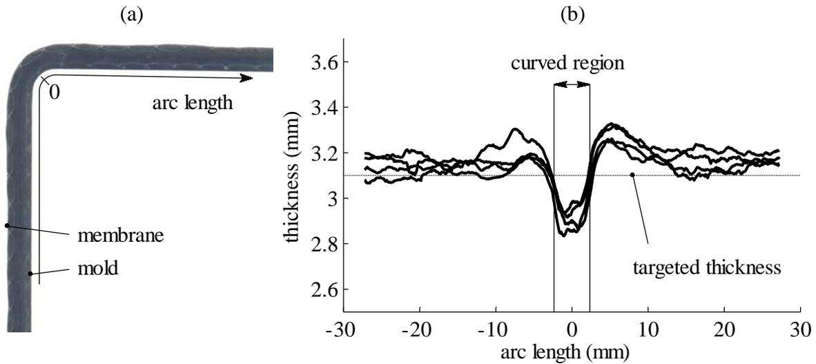
Fig. 6 Analysis of parts fabricated with preform A: (a) typical cross-section and (b) thickness profiles.
