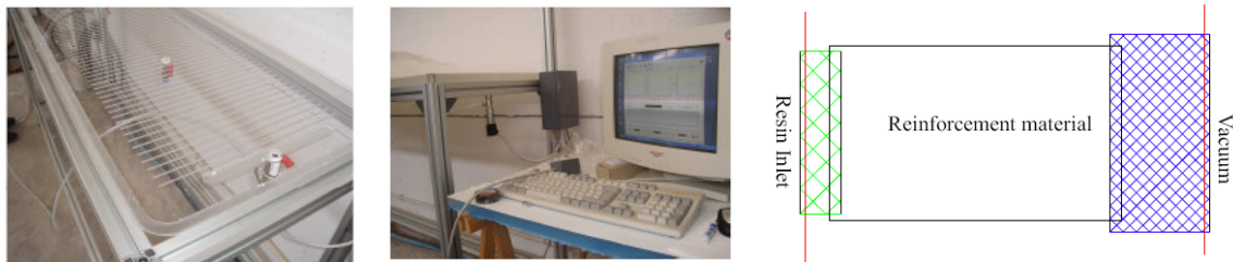
Figure 2.- Experimental set-up for 1D flexible permeability measurement
