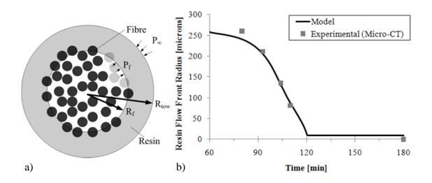
Fig. 3 a) Schematic of fibre tow approximation; b) graph of resin flow front radius versus time from experiments and modeling.
