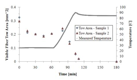
Fig. 2 Visible fibre tow area and cure cycle temperature with processing time.
