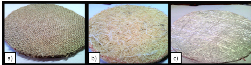
Fig. 1 Reinforcements used in the compaction tests. a) Jute woven Fabric, b) Sisal fiber Mat, c) Glass fiber mat.
