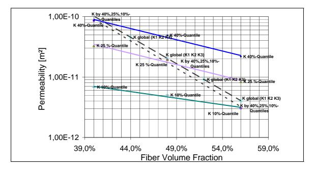
Fig. 3 Plot of the global permeability (as displayed in Figure 1) and the 10 %-, 25 %and 40 %-quantiles. The dotted line is built up of the following interpolation points: the permeability value calculated from the 40 %-quantile at a Vf of 40%, the permeability value calculated with the 25 %-quantile at a Vf of 48 % and to the permeability at a Vf of 56 % the 10 %-quantile.
