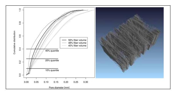
Fig. 2 left: Plot of the cumulative pore volume distribution versus pore diameter, continuous lines are the average, dotted lines are single samples. This plot makes it possible to read out quantiles. right: Image of the analyzed resin structure, the fibers are subtracted of the glass fiber reinforced epoxy image.
