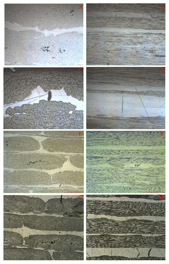
Fig. 3 A 30 x optical micrograph of polished and unpolished cross-section of a G/CBT symmetric and unidirectional laminates  $(1^{st} \text{ and } 2^{nd} \text{ row unpolished and polished unidirectional G/CBT; } 3^{rd} \text{ and } 4^{th} \text{ row unpolished and polished symmetric G/CBT NCF})$
