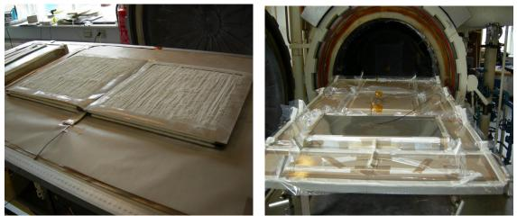
Fig. 1 Lay-up and the oven (in this case an autoclave) used for the vacuum consolidation process
