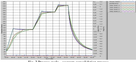
Fig. 2 Process cycle - vacuum consolidation process
