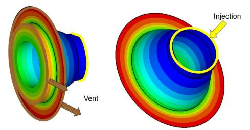
Figure 5: The results of the flow simulation for the output housing. Different colors indicate different times of resin arrival.
