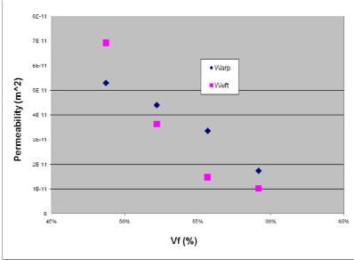
Figure 2: The permeability of the fabric
