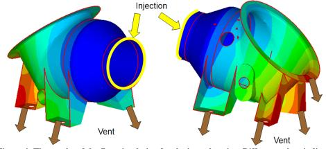
Figure 4: The results of the flow simulation for the input housing. Different colors indicate different times of resin arrival.
