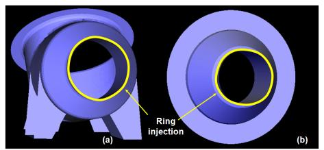
Figure 3: The proposed injection locations for (a) the input and (b) the output housings
