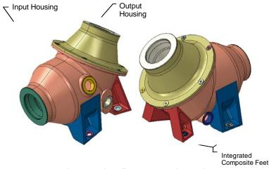
Figure 1: Final Gearbox Housing Design
