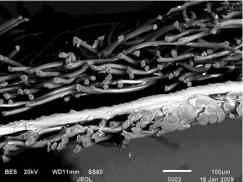
Figure 1: A section through a typical trilaminate separator layer. (Image acquired by the University of Plymouth Electron Microscopy Centre).
