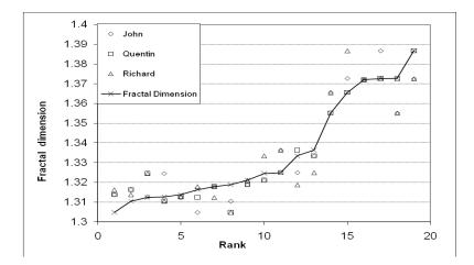
Figure 5: Correlation of the fractal dimension and human assessment of gel coat quality
