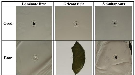
Figure 2: Photographs of typical in-mould gel-coated laminate surfaces for 10% fibre volume fraction composites. The central defect arises from the position of the gel-coat inlet gate.
