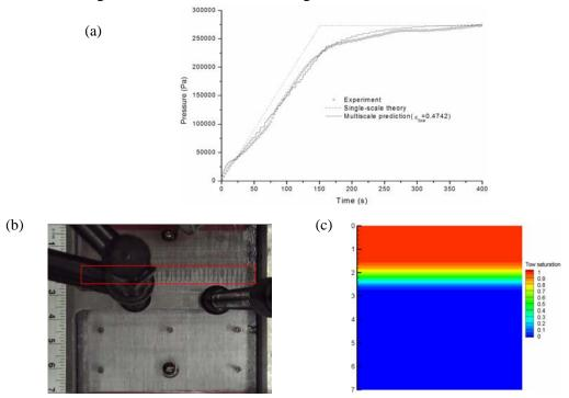
Figure 5: (a) Comparison of the experimental inlet-pressure history with the numerical predictions; (b) tow-saturation distribution from the experiment at 67s; (c) tow-saturation distribution from the multiscale prediction at 67s.
