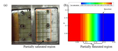
Figure 3: Snap shots of the tow-saturation distributions at t = 24s during the 1-D flow experiment: (a) from the experiment; (b) from the dual-scale mold-filling simulation.
