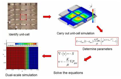
Figure 1: the lumped algorithm of modeling dual-scale flow in LCM
