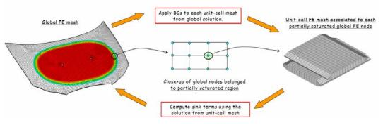
Figure 4: Relation between the global and local unit-cell FE models.
