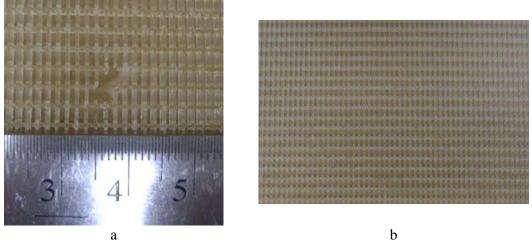
Figure 5. Reference media: a) a damaged and deformed reference medium, b) a reference medium in sound condition
