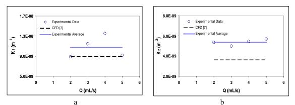
Figure 4. Comparison of the experimental results obtained using the 1-D transient-filling experiments with the CFD simulation results obtained from [7] for the principal permeabilities  $K_1$  and  $K_2$ .
