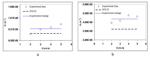
Figure 3. Comparison of the experimental results obtained using the 1-D steady-state experiments with the CFD simulation results obtained from [7] for the principal permeabilities  $K_1$  and  $K_2$ .
