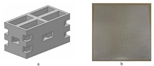
Figure 1. Detailed view of a) unit-cell structure suggested by Morren et. al [6], b) reference porous-medium made by rapid prototyping.
