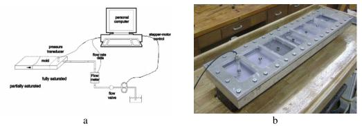
Figure 2. Experimental setup: a) schematic view; b) 1-D flow experiment setup
