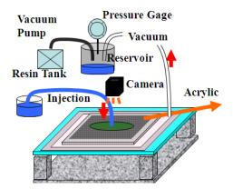
Fig.3 Experimental equipment.
