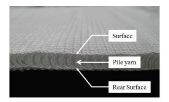
Fig.1 3-D hollow knitted fabric before resin impregnation
