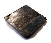
**Figure 1:** Picture of a specimen after squeezing. The dots on the surface were marked prior testing to determine whether the material slips at the walls.
