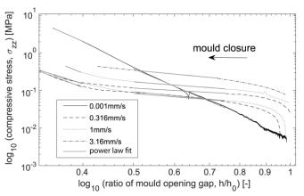
Figure 2: Experimentally observed axial stress vs. mould opening.
