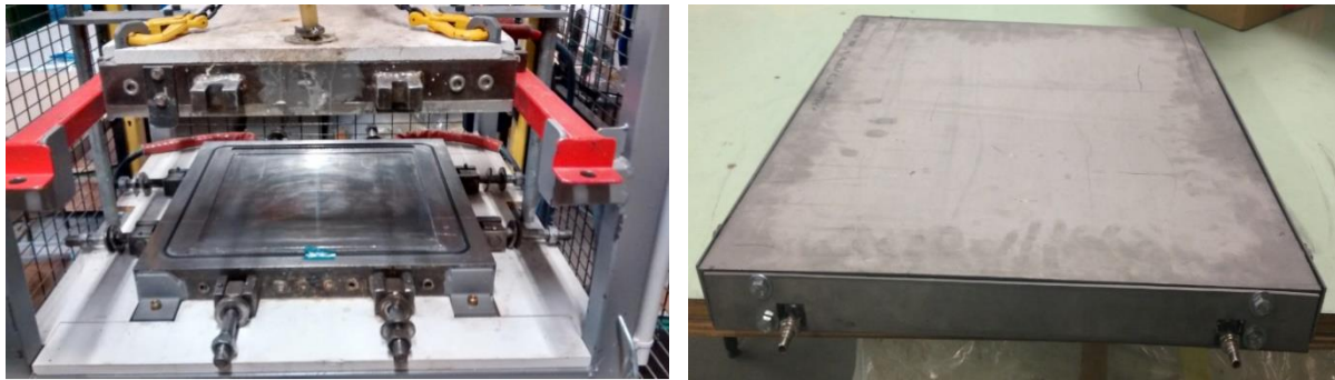
Figure 1: Massive reference RTM mold (left) and innovative low inertia mold with rectangular heating channels (right).
