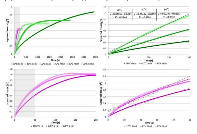
Figure 1: Wicking in quasi-UD carbon fabric along the fibres main direction with silicon oil and epoxy resin.
