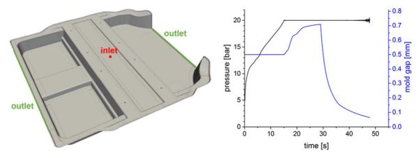
**Figure 3:** Left: geometry of the application example; Right: Simulation results of pressure and mold gap during mold filling; mold gap at the beginning 0.5 mm; injection time 29 sec; maximum pressure 20 bar.
