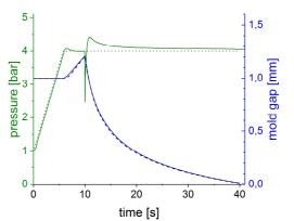
**Figure 2:** Comparison of a PC-RTM simulation (continuous lines) with an analytical solution of a onedimensional Darcy-equation (dots).
