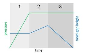
**Figure 1:** Schematic representation of inlet pressure and gap height of a PC-RTM process with three stages; 1: Injection with constant mold gap; 2: Injection with a pressure controlled increase of the mold gap; 3: Pressure controlled compression to final part thickness.
