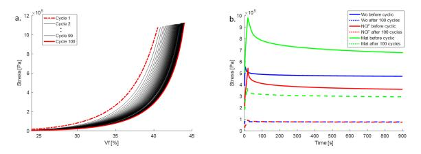
Figure 1: Cyclic compaction curves (Mat textile) (a). Final compaction step before and after preconditioning (b).
