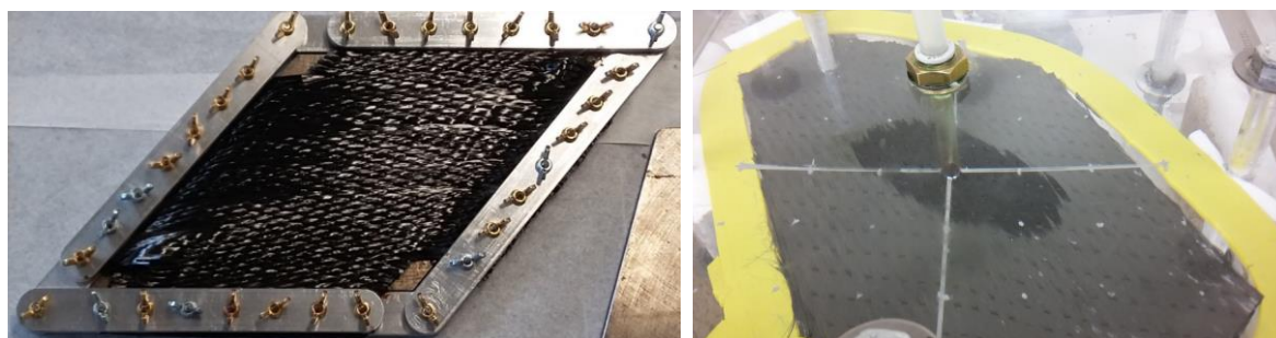
Figure 3: Shear trellis tool (left) and three-dimensional permeability test with the sheared sample (right).
