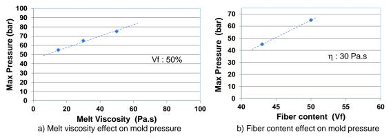
**Figure 1:** Evolution of max pressure P (compression) with melt viscosity  $\eta$  a) and fiber content Vf b) PA6 and plain glass preform system
