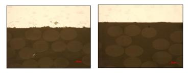
Figure 1 : Micrographs of Elium© 150/GF & Aluminium: HCl Surface treatment (left); Silane based coating (right)
