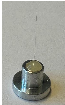
Single Fiber Pull Out Specimen
