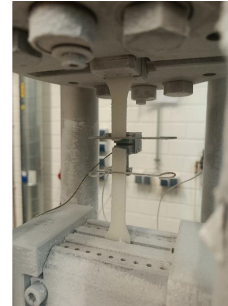
Figure 2: Tensile strength test at 77 K in LN2
