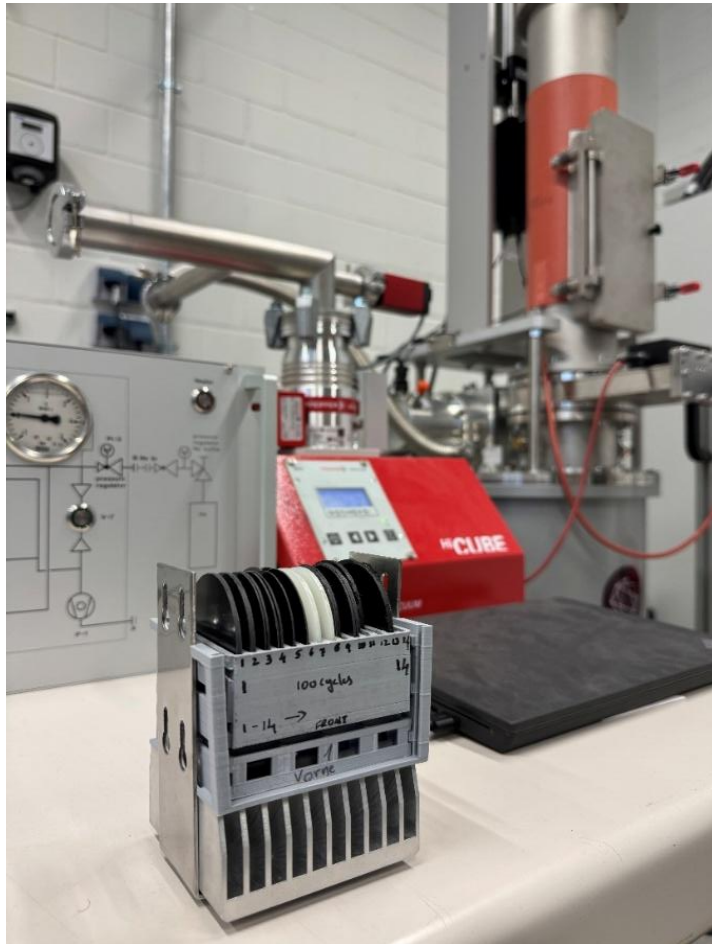
Figure 1: Specimen holder & cryogenic cycling system
