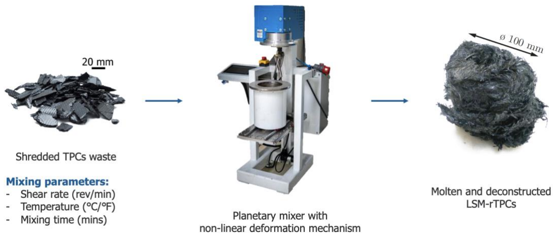
Figure 1. Recycled thermoplastic composites (rTPCs) from low-shear mixing (LSM) process
