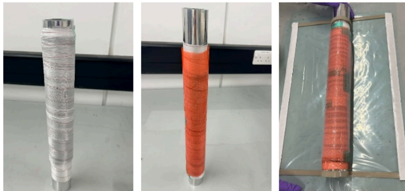
Figure 2: Preparation of the vacuum bag for VARI
